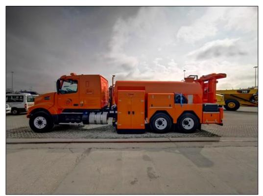
WDM's SCRIM® combines continuous pavement friction measurement with GPS-linked texture, IRI, and geometric data to provide critical insight into friction's role in road performance.
